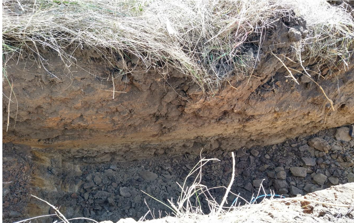
Photo 5: Test Pit 107 profile (refusal at 1.1m) Typical of northern part of Stage 2
