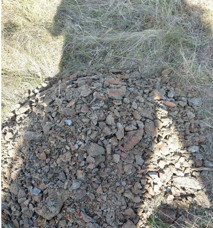
Photo 8: Medium to low strength shale from base of Pit 117
